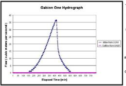
This graph is the hydrograph generated from Gabion One. The blue curve shows the inflow to the gabion. The lack of a second curve indicates that. with a 111.4 mm storm, there is no outflow from aabion farthest downstream when represented alone.
